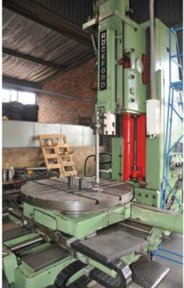
The Rockford vertical slotter is capable of machining components with an outside diameter 2000 mm and a 1000 mm height
